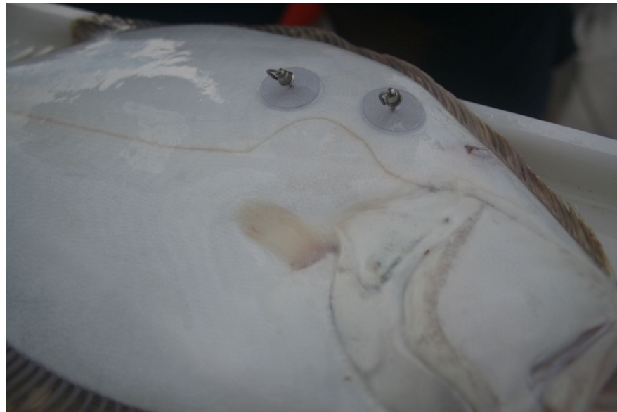
Figure 2. (A) Placement and orientation of the externally attached Star-Oddi DST milli-L archival tag on a 436 mm TL summer flounder. (B) plastic discs and earring backings used on the non-pigmented side of the fish to secure the archival tag.
