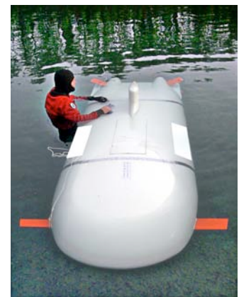
ASL personnel have designed and built larger AUVs. This vehicle has a 500 lb payload capacity, and active buoyancy control. Prizm, a commercial AUV manufacturer, is a founding sponsor of the ASL.
