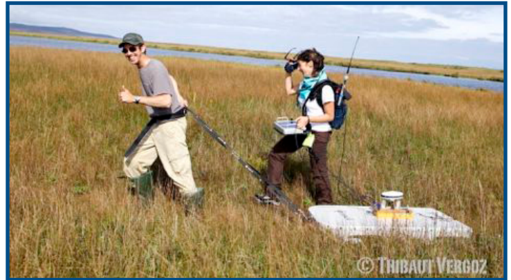
Ground Penetrating Radar: Chris Hein and Julie Billy of the University of Perpignan use a ground-penetrating radar unit to investigate the beach-ridge plain of the Miquelon-Langlade Barrier in France. © Thibaut Vergoz / CNRS Images
