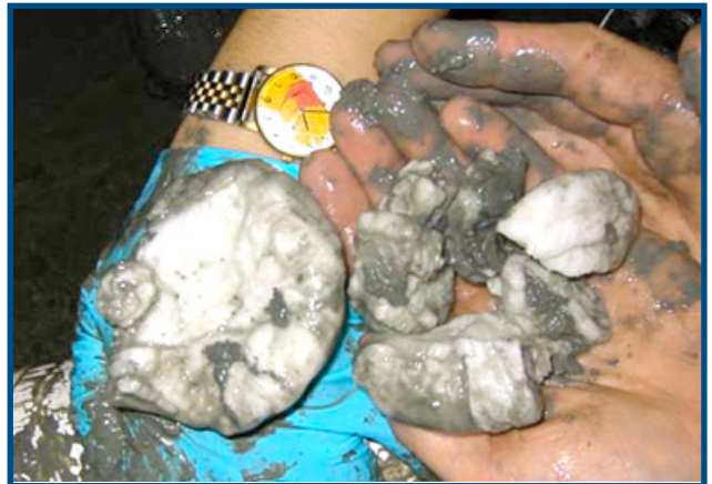
Gas Hydrate: Chunks of gas hydrate recovered from the Gulf of Mexico in 2002. Photograph by Bill Winters, USGS.
