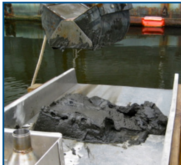
The type of sediment grab used to collect samples for the study. Photo by Mike Unger
